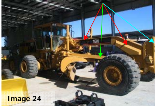
Image 24: The Gooseneck (red arrows), circle arms (green arrow) and front end (Aqua arrow) of the Grader.
