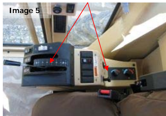
Image 5: All joystick control panels will need to be cleaned internally and be accessible at the time of inspection.
