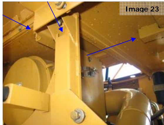
Image 23: Further illustrations of the hollow support framework that may be located under engine cover covers.
