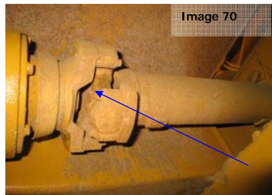
Image 70: All contaminated grease is to be removed from all universal joints.
