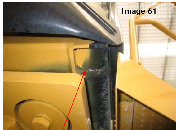
Image 61: Underneath the cabin, the framework may be open-ended as illustrated (small triangular corners missing) and will require flushing to verify cleanliness.
