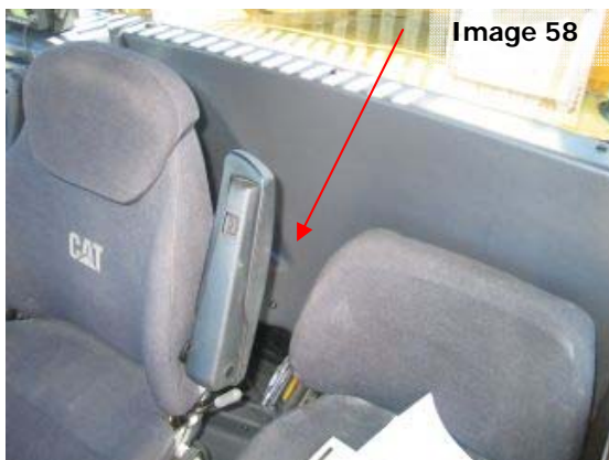
Image 58: Verify behind all internal cabin wall linings is free of contamination.
