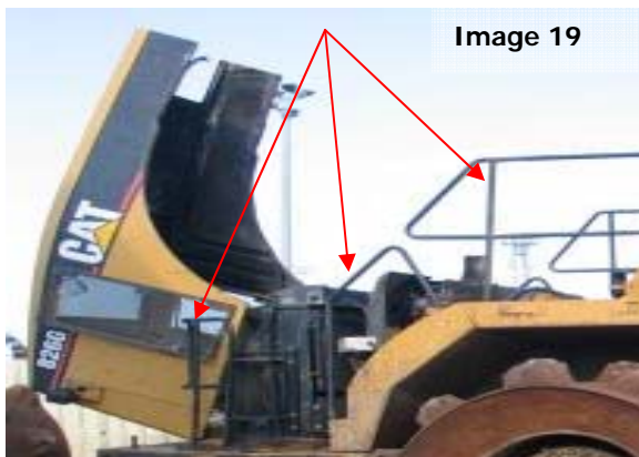
Image 19: Some engine covers may tilt rearwards as illustrated, exposing the topside of the engine block. The engine covers must be checked for hollow rails and flushed if present. Check all handrails (red arrows) for open ends or drainage holes that can be flushed.
