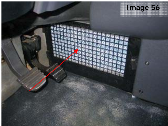
Image 56: Remove the air-filter cover (red arrow) and verify the cleanliness of the filter (pressurised air).
