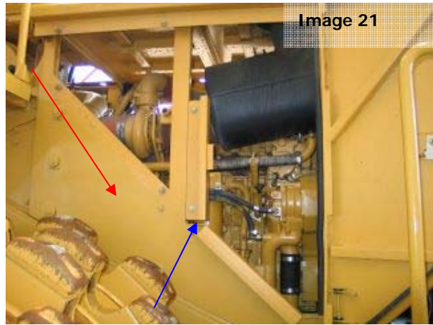
Image 21: A fixed Compactor engine housing will non-affixed panels (red arrow) and hollow framework (blue arrow).
