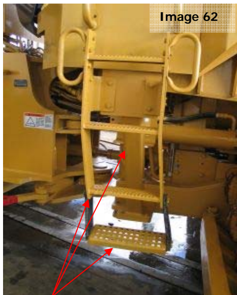
Image 62: Check all footsteps for cleanliness (including underside).
