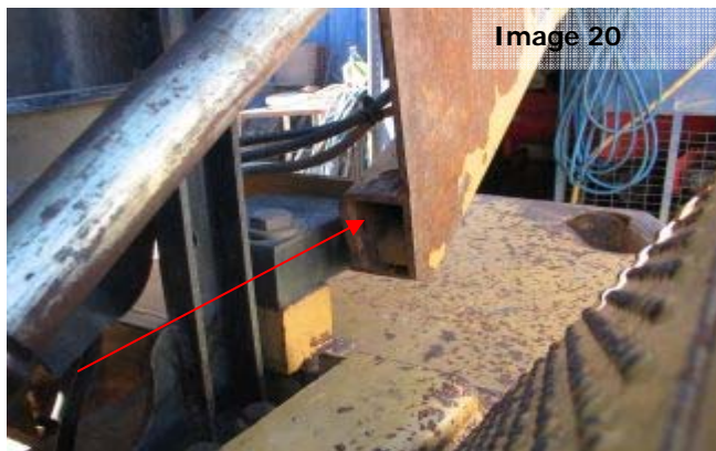
Image 20: An illustration of a hollow channel in the engine cover (red arrow) of the Compactor. This will require flushing to verify cleanliness.
