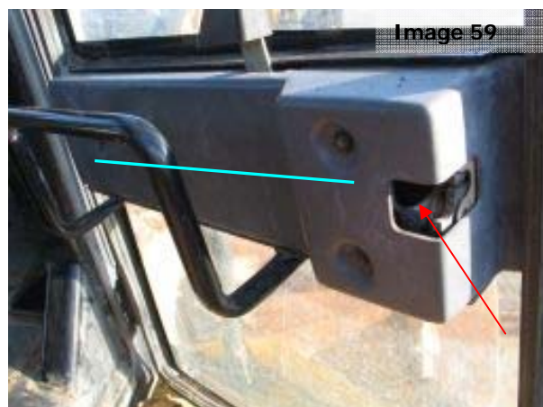
Image 59: The door latches are hollow structures and verification of internal cleanliness is required.
