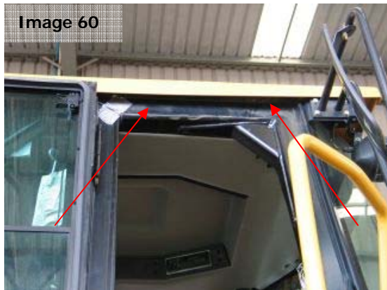
Image 60: On some models a small recess can be found between the cabin roof and the Roll Over Protection System (ROPS).
